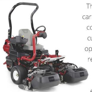
The new Greensmaster® eTriFlex models carry no hydraulic fluid and utilize all-electric components for traction, steering, lift and cutting. These EnergySmart® models are operationally friendly with noticeable noise reductions, operational cost savings, and other meaningful improvements to complement the ever-important enhancements in cutting performance.
